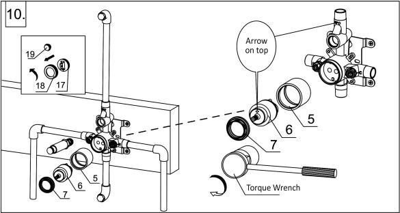
Remove the pipe plug (19), switch nut (18), and diverter plug (17) again. Install the cartridge cover (5), cartridge (6), and cartridge nut (7) into the valve main body. When installing the cartridge (6), make sure the arrow is on top pointing toward the valve. Use a torque wrench (10-12 Nm) to assemble. Turn the valve clockwise to the open position to test for tightness: water pressure should be at or less than 1.6 Mpa when open and 0.4 Mpa when closed.
