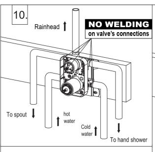
Connect to the hot and cold water supplies and outlets to test the tightness. Water pressure should be at or less than 1.6MPa (145psi) when opened and should be at or less than 0.4MPa (58psi) when closed.
